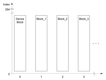
There are 254 indices per slot. The indices can have a width of 255 bytes. All values that can be accessed via Profibus have to be mirrored to one of these slots/indices
