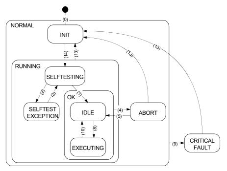
After the start, the gauge independently runs through the INIT and SELFTESTING status and eventually changes to the IDLE status (if there is no error) or to the SELFTEST EXCEPTION status (if there is a gauge error).
