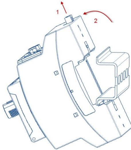
*Fig. 7: Removing the I/O module*
