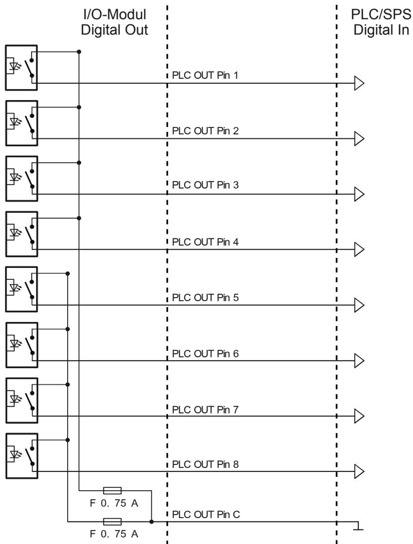
Fig. 3: Sample wiring, digital outputs
