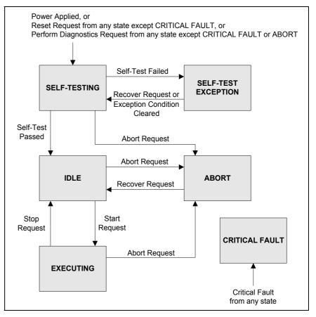
**Abort** - Used to transition the device application objects to the aborted state. This service request may be (and generally will) originated internally, from application objects.
