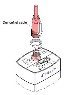
3 Lock the DeviceNet (and sensor) cable connector.
