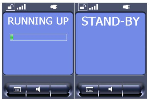
Fig. 27: "Running up" and "Stand-By" status displays
