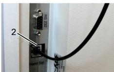
Fig. 3: Connecting radio transmitter and leak detector (RC1000WL)
