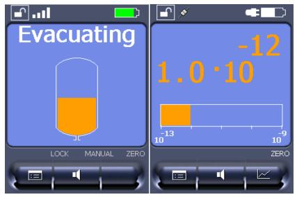
Fig. 28: "Evacuating" and "Measure" status displays (numerical and bar graph)
