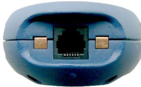
Fig. 4: RJ25 socket on the bottom of the remote control
