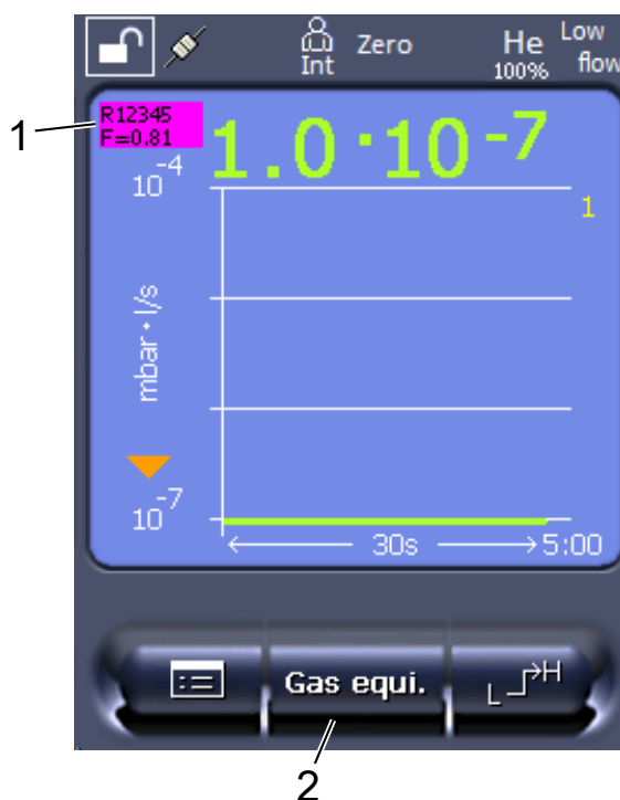
Fig. 3: Measurement screen with displayed equivalence leak rate and configured favorites key
