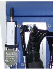
Fig. 21: Fasten the transmitter with Velcro in a free place
