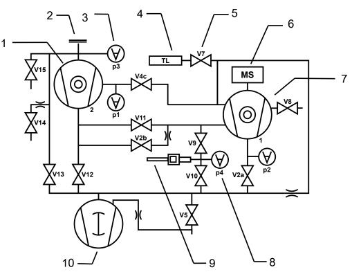
Fig. 13: UL6000 Fab: Main components of the vacuum diagram
