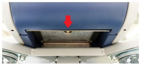
**3** Remove the metal sheet with the filter mat. The metal sheet can be pulled out more easily by holding it in an inclined position.
