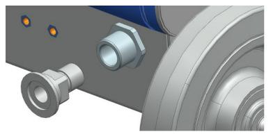
• If you have an exhaust hose with a hose nozzle (G <sup>1</sup>/<sub>2</sub> inch male thread), you can alternatively fix this hose nozzle in the exhaust port by turning it clockwise.
