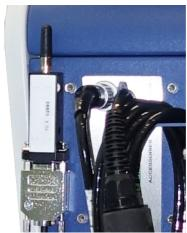
Fig. 20: Fasten the transmitter with Velcro in a free place
