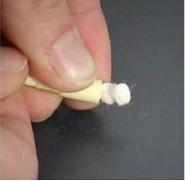
Fig. 17: Pressing the filter inserts out of the capillary filter
