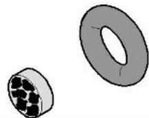
Fig. 17: Sintered filter heavily soiled
