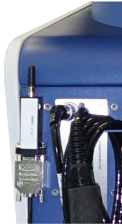
Fig. 22: The transmitter can be attached to a free spot with the supplied Velcro tape.
