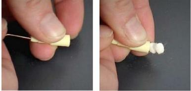
Fig. 19: Pressing the filter inserts out of the capillary filter
