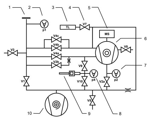
Fig. 15: The most important components of the vacuum diagram in UL3000 Fab PLUS devices
