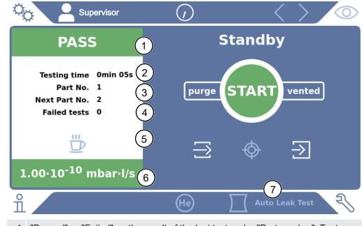
1 "Passed" or "Failed" as the result of the last test under "Part number". Test failed if the leak rate exceeds the setpoint.
