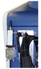
*Fig. 22:* The transmitter can be attached to a free spot with the supplied Velcro tape.
