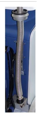
Fig. 9: The bracket for corrugated tube is mounted.
