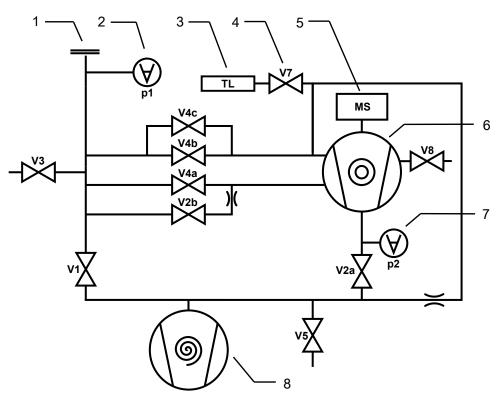
Fig. 14: The most important components of the vacuum diagram in UL3000 Fab devices
