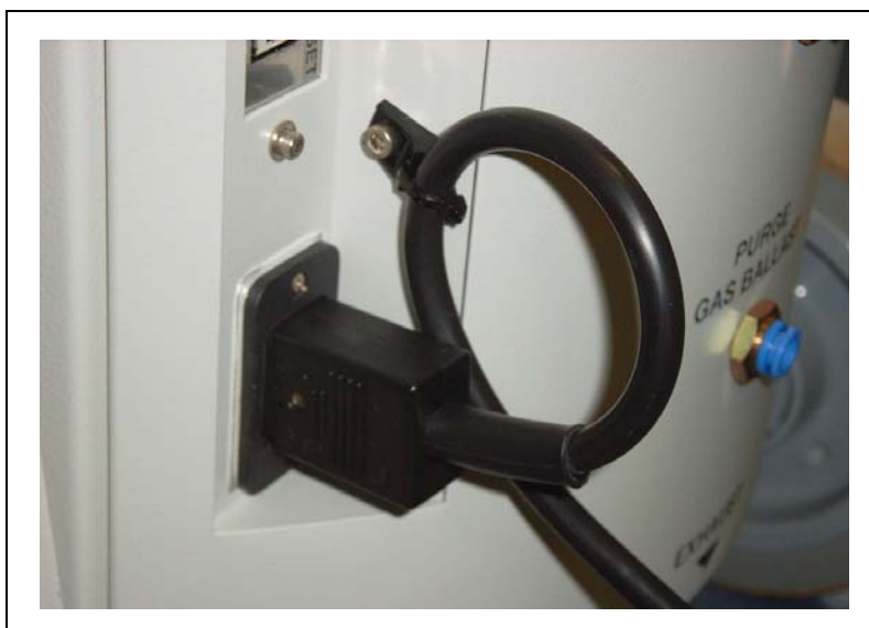
Fig. 2-4 secure fixture power cord
