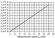
$$p = [(I_{out} - 4 \text{ mA}) / 16 \text{ mA}] \times p (F.S.)$$
