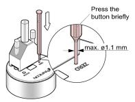
... briefly apply the supply voltage to pin 6 (Remote Zero,  $(\rightarrow \text{diagram} \ \mathbb{B} \ 16. \text{ pulse} \rightarrow \mathbb{B} \ 9).$
