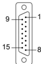
D-sub, 15-pin female soldering side
