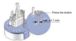
For changing the threshold value, push the <ZERO> button and keep it depressed. The threshold keeps changing from the current value (ramp) until the button is released or until the limit of the setting range is reached.
