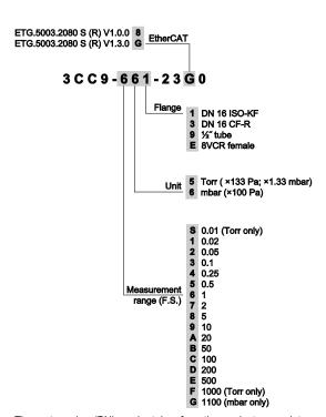
The part number (PN) can be taken from the product nameplate. If not indicated otherwise in the legends, the illustrations in this document correspond to gauges with DN 16 ISO-KF vacuum connection. They apply to gauges with other vacuum connections by analogy.
