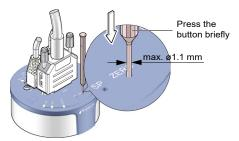
... apply supply voltage to Remote Zero at pin 10 (pulse  $\rightarrow \mathbb{B}$  11).
