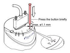
After zero adjustment, the gauge automatically returns to the measurement mode.
