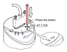
Por changing the threshold value, push the <ZERO> button and keep it depressed. The threshold keeps changing from the current value (ramp) until the button is released or until the limit of the setting range is reached.
