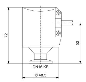
Fig. 1 Dimensional diagram VSA100A
