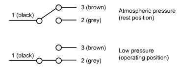
Fig. 2 Contact assignment of microswitch
