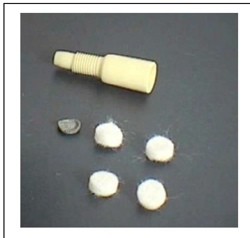
Fig. 8-10 old and new filter pads
