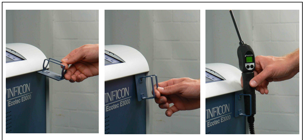
Fig. 1-6 Installation of sniffer line holder
