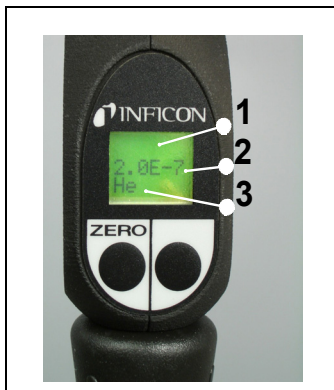
Fig. 3-5 Sniffer display in standard operation mode
