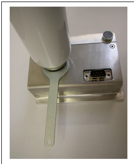
Fig. 8-18 Installing the gas reservoir
