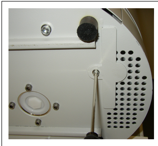
Fig. 8-1 Fastener for the air filter on the bottom of the Ecotec E3000
