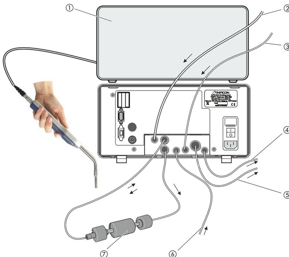
Fig. 10: Example of a test setup with an elongated test object
