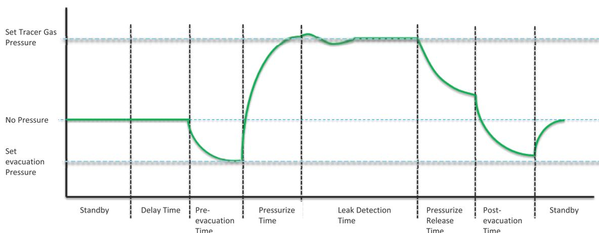
Fig. 6: Time pressure diagram Mode A
