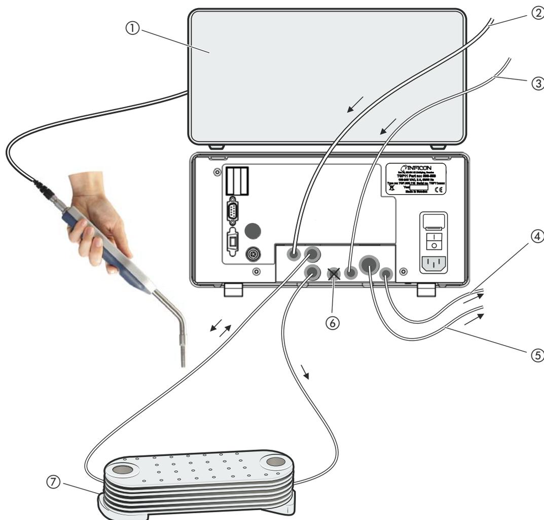
Fig. 9: Setup of the tracer gas filling the test object with gas via test port 1 and 2
