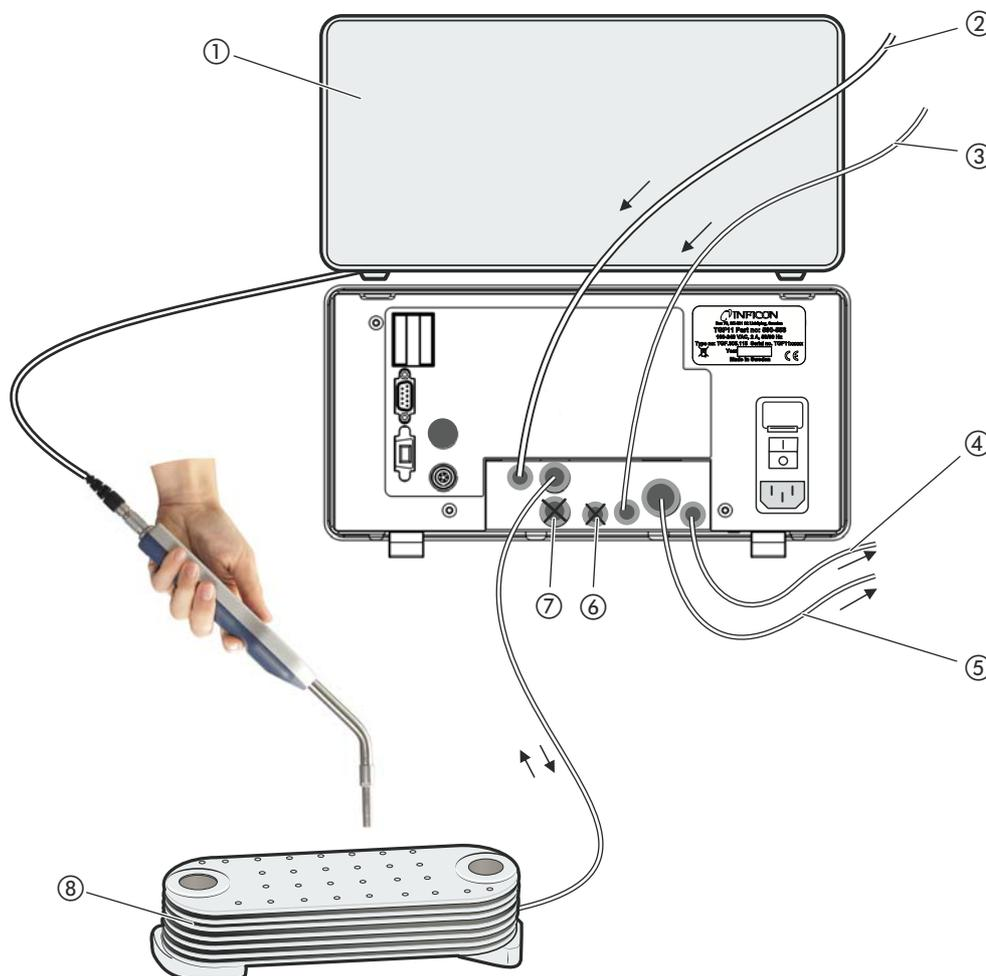
Fig. 8: Setup of the tracer gas filling unit if the test object is to be single fed.
