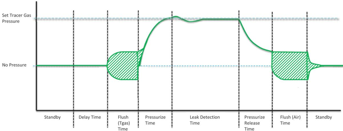
Fig. 7: Time pressure diagram Mode B
