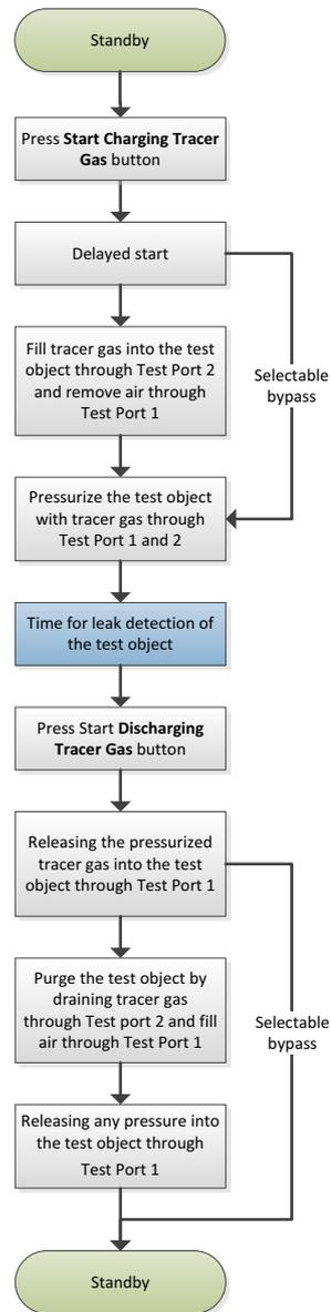
Fig. 3: Flowchart Mode A versus Mode B
