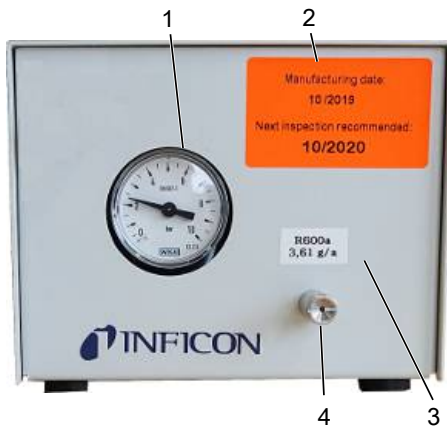
Fig. 1: Test leak without proof
