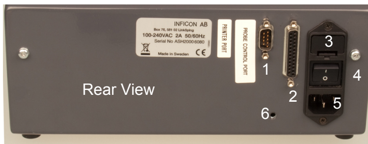
Fig 3-2. Sensistor ISH2000 ports and connections.
