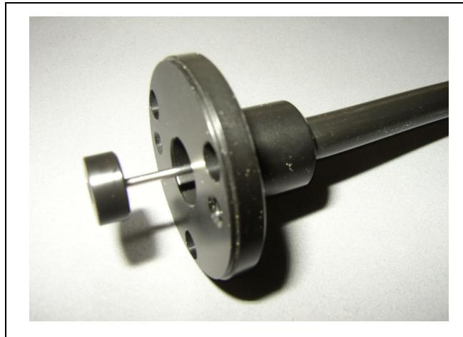
Fig. 82 Steel capillary sticking out of sniffer tip flange
