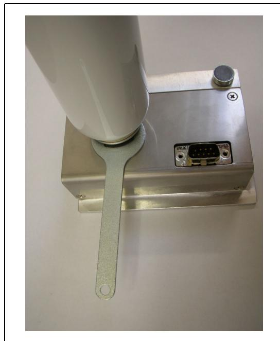
Fig. 85 Installing the gas reservoir
