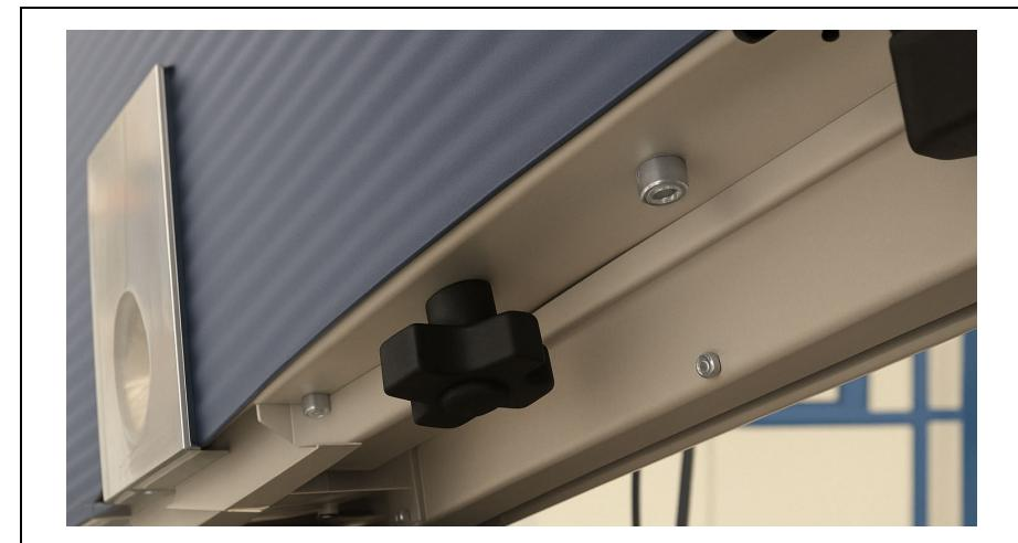
Fig. 2 *Removing the transportation lock before starting*
