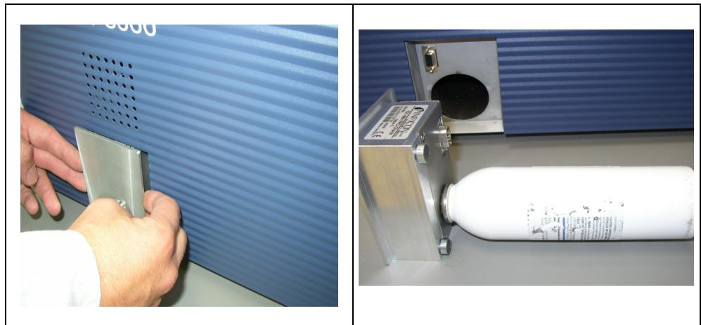
Fig. 83 Removing the PRO-Check reference leak from the main unit
