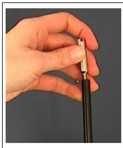
Fig. 3 *Installing water protection tip*
