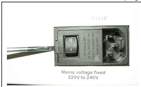
**2** Pull out the two slots and replace both fuses.
