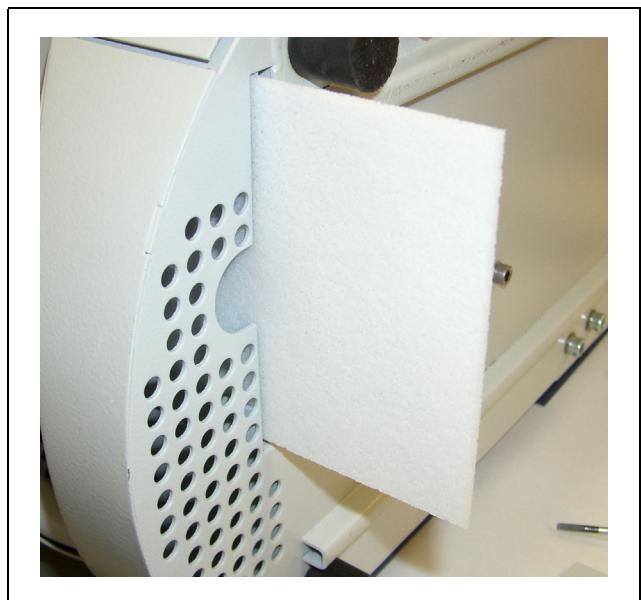
Fig. 70 Inserting the air filter
