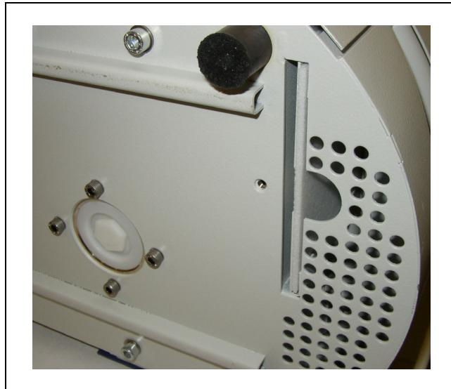
Fig. 69 Dismounting of the air filter
