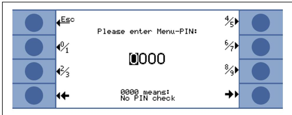
Fig. 52 Setting-up a Menu-PIN for parameter protection
