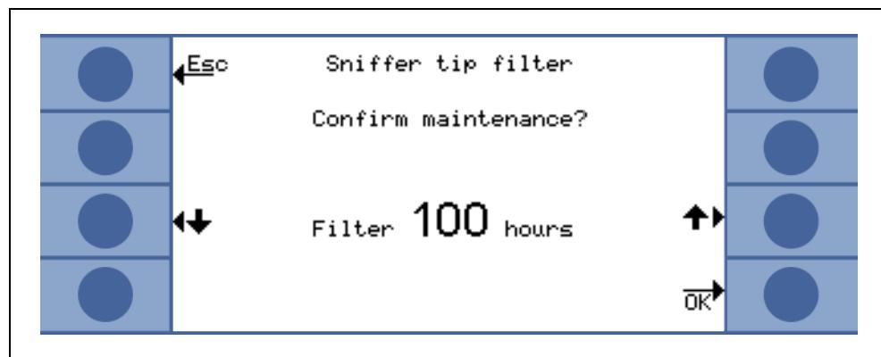
Fig. 60 Setting the maintenance interval for the sniffer tip filter and confirming its replacement
