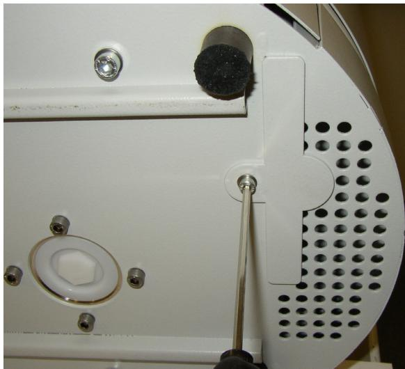
Fig. 68 Fastener for the air filter on the bottom of the leak detector
