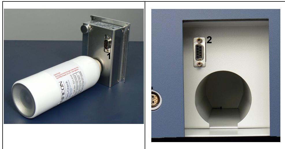
Fig. 15 Connections for remote use
