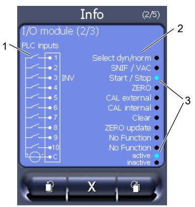
Fig. 21: I/O module (2): Visualized information to the digital inputs
