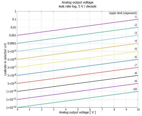
Fig. 19: Analog output voltage leak rate log. 5 V / decade
