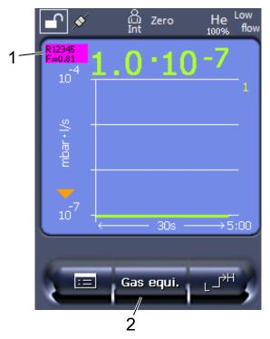
Fig. 23: Measurement screen with displayed equivalence leak rate and configured favorites key
