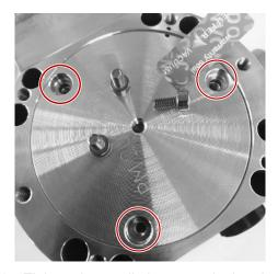
6 Tighten the ventilation screw by hand.
