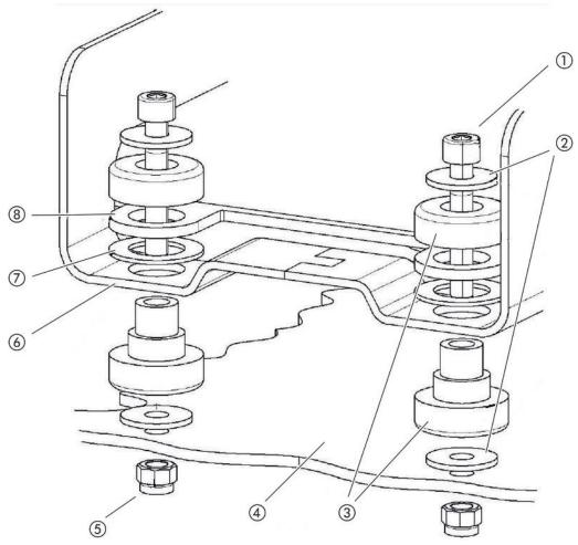
Fig. 11: Components of a fastener
