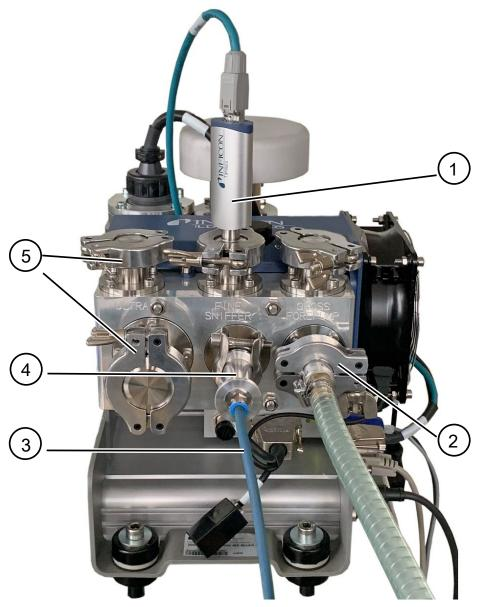
Fig. 3: Mass spectrometer module (execution accumulation)
