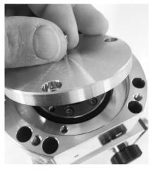
5 Screw in the 3 screws (M4) of the cover with the Allen key and a torque of 3 Nm.
