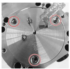
**3** Screw a threaded screw (M5) a few turns into the empty central threaded opening of the aluminum cover.
