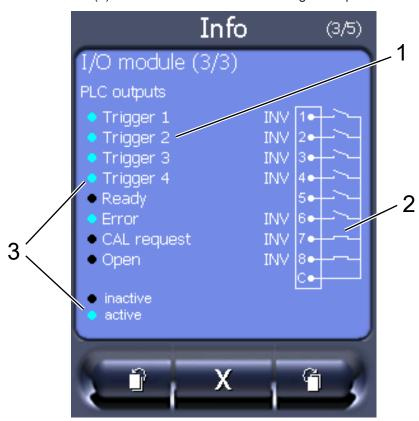
• I/O module (3): Visualized information to the digital outputs
