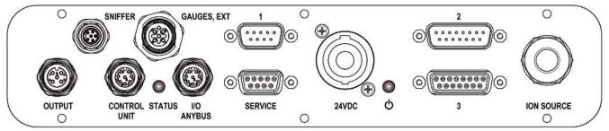
Fig. 7: MSB box connections
