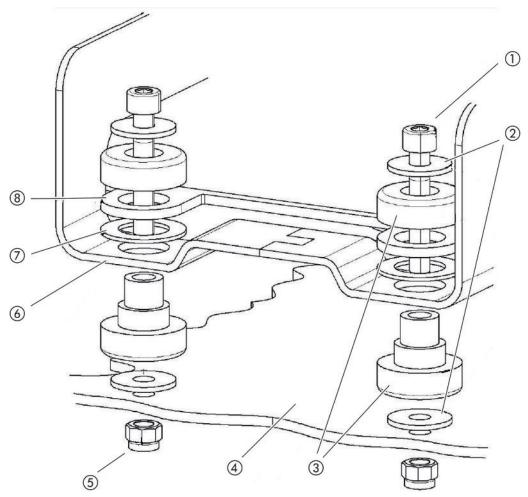
Fig. 9: Components of a fastener
