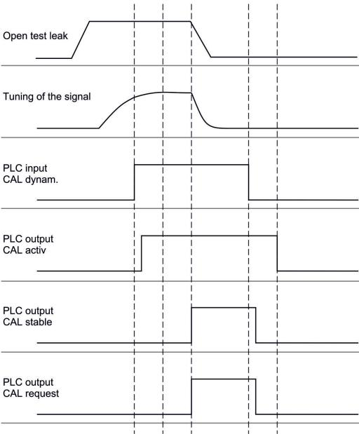
Fig. 15: Fig. 7 External dynamic calibration with IO1000 using the example of sniffer line SL3000XL, description of PLC inputs and outputs: "Assigning inputs and outputs [ 97]"
