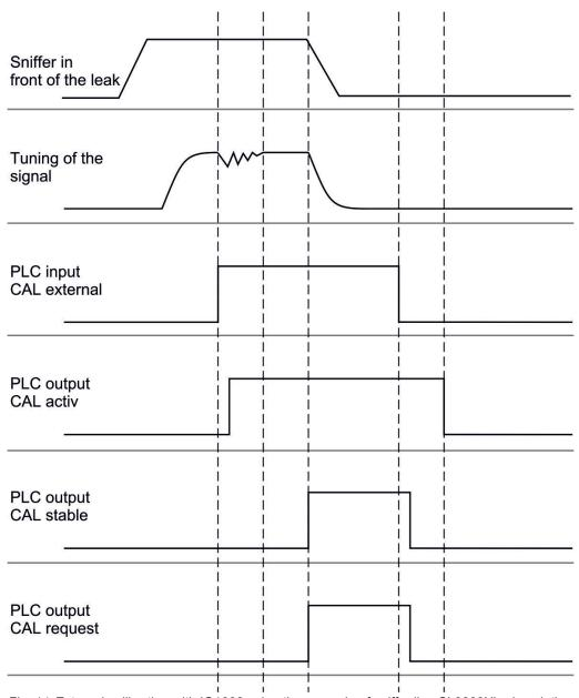
Fig. 14: External calibration with IO1000 using the example of sniffer line SL3000XL, description of PLC inputs and outputs: "Assigning inputs and outputs [ $\triangleright$  97]"
