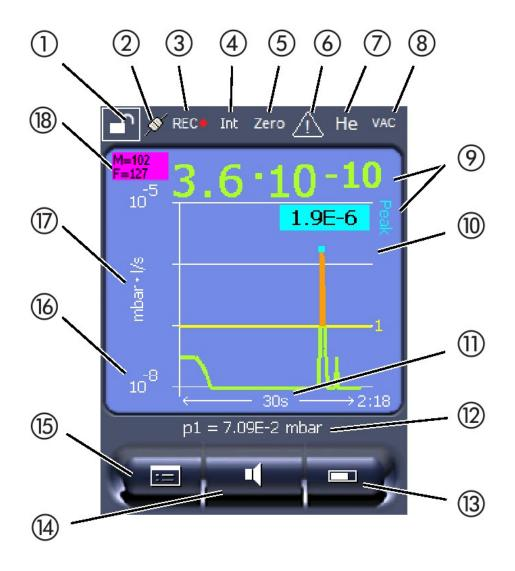
Fig. 20: Measurement display
