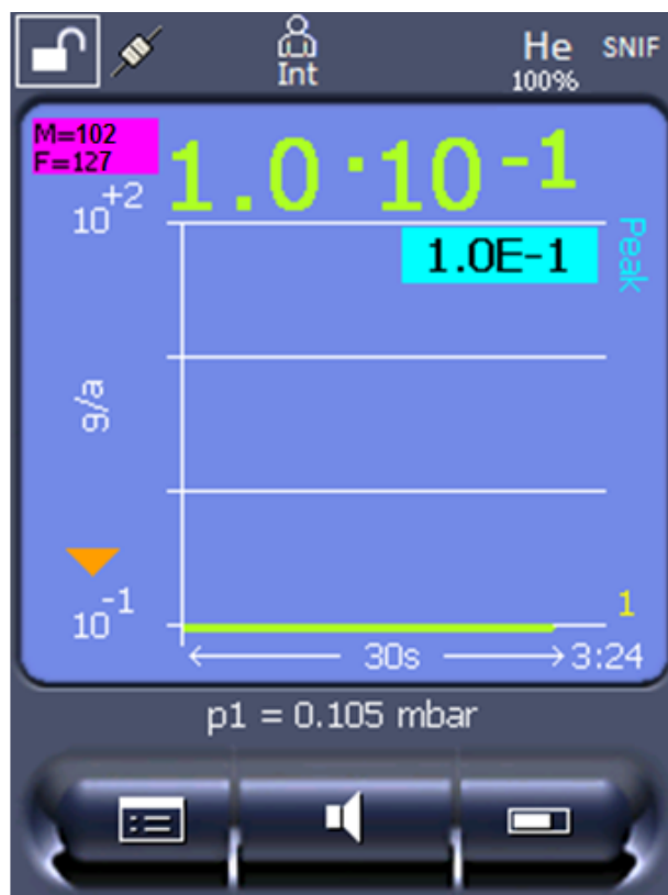
Fig. 15: Top left: Display of Molar Mass (102) and Equivalence Factor (127)
