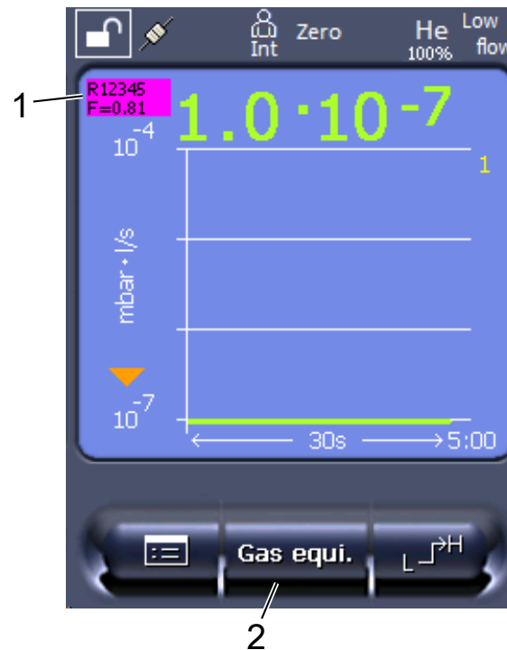
Fig. 14: Measurement screen with displayed equivalence leak rate and configured favorites key
