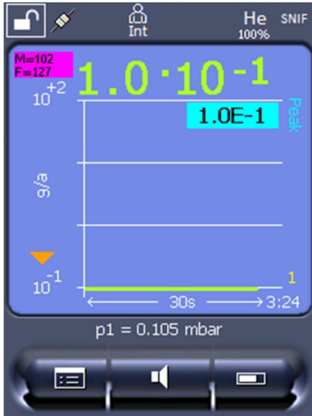
Fig. 24: Top left: Display of Molar Mass (102) and Equivalence Factor (127)
