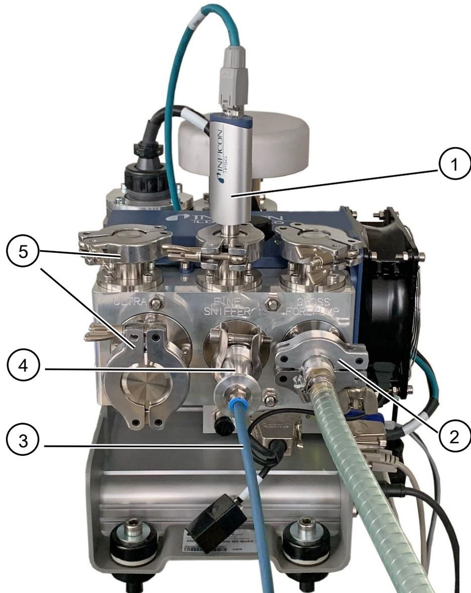
Fig. 3: Mass spectrometer module (execution accumulation)
