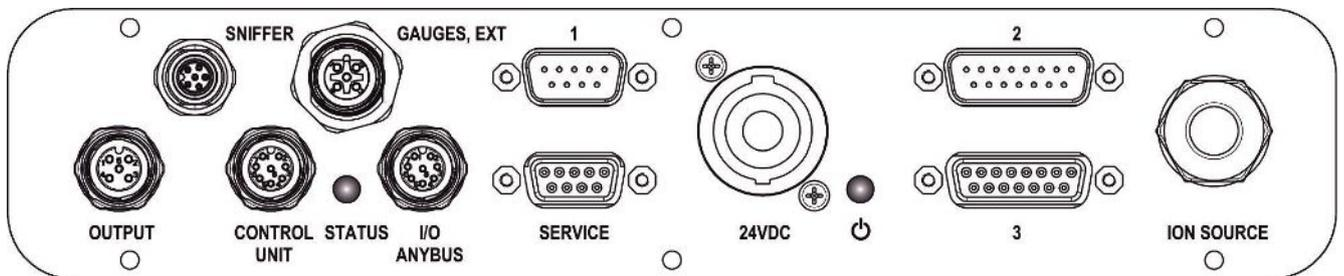
Fig. 7: MSB box connections
