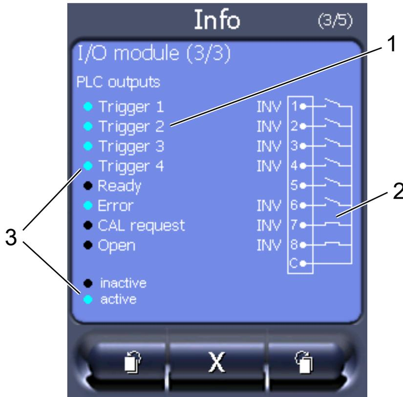
Fig. 22: Visualized information to the digital outputs
