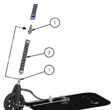
Fig. 12: Assembling the probe system 3
