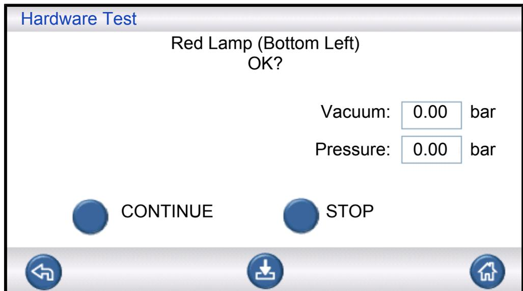
This is a “manual” test. The ILS500 F/FHP lights up one lamp at the time. Simply check that the right lamp comes on.
