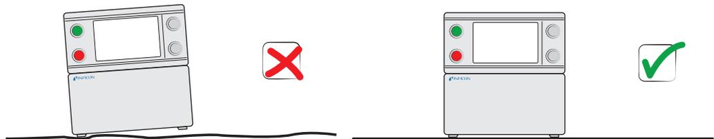
Place the ILS500 F/FHP on a flat surface, as close as possible to the test fixture and ventilation system.
