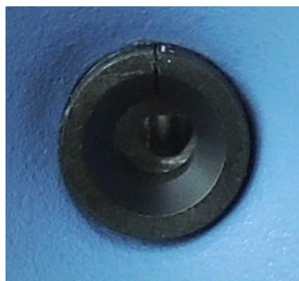
Fig. 10: Insert centering ring
