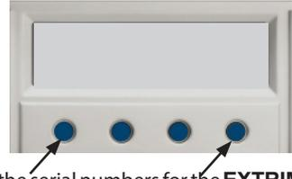
During warm up the display will show software versions and the serial numbers for the **EXTRIMA** and the Hand Probe PX57. Time and the inside temperature are also shown. All menu items, except showing the service mode display, are locked by a password.
