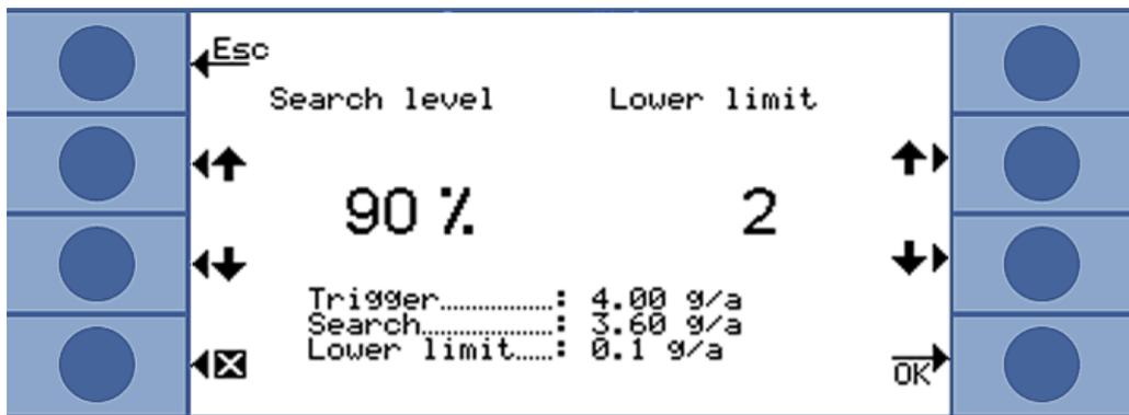
Fig. 23: Setting display limit and search threshold
