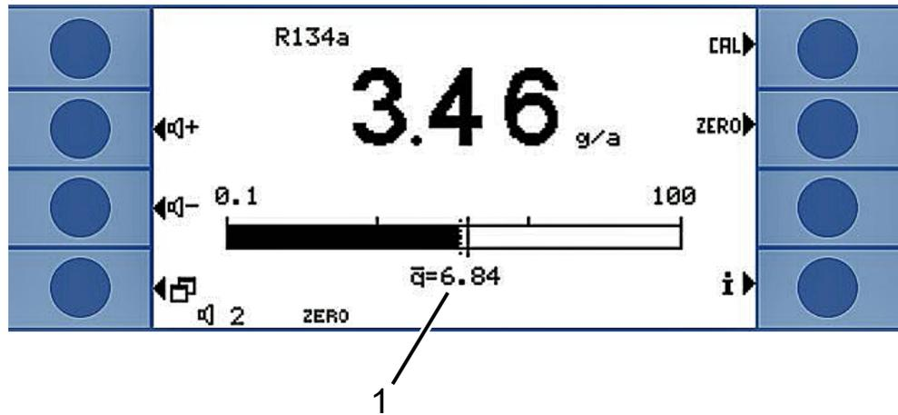
Fig. 15: Measurement view with maximum value display
