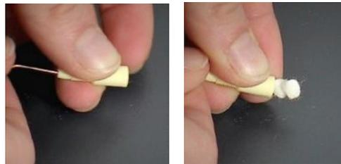
Fig. 53: Pressing the filter inserts out of the capillary filter
