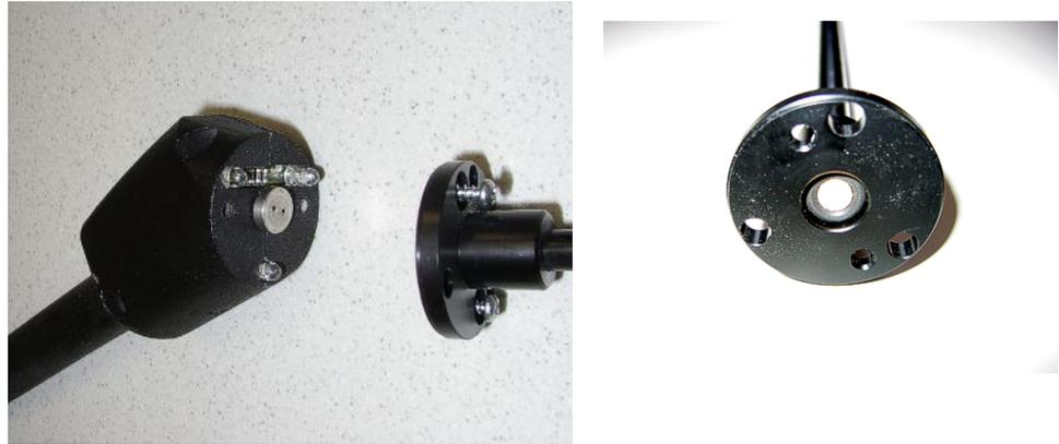
*Fig. 54: Sinter filter in the sniffer handle*
