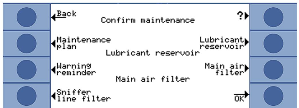
Fig. 43: Confirming maintenance work
