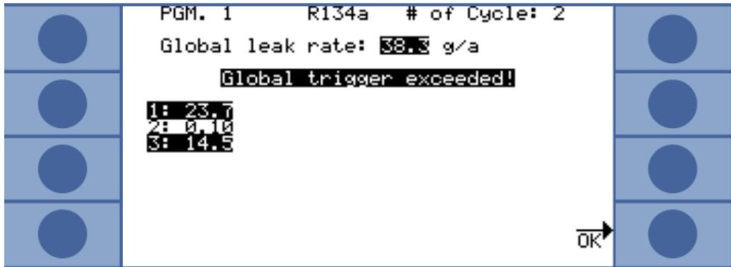
Fig. 36: Search with I•Guide-Program 1 for gas R134a: The trigger value and the total leakage rate were exceeded at measuring points 1 and 3.
