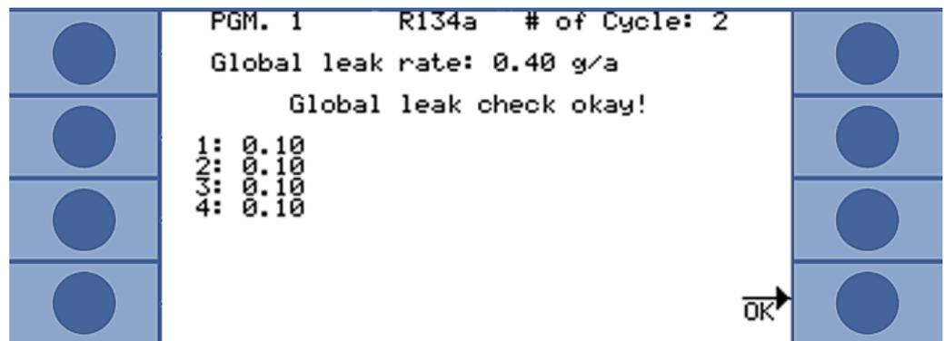
Fig. 35: Display after a successful measurement
