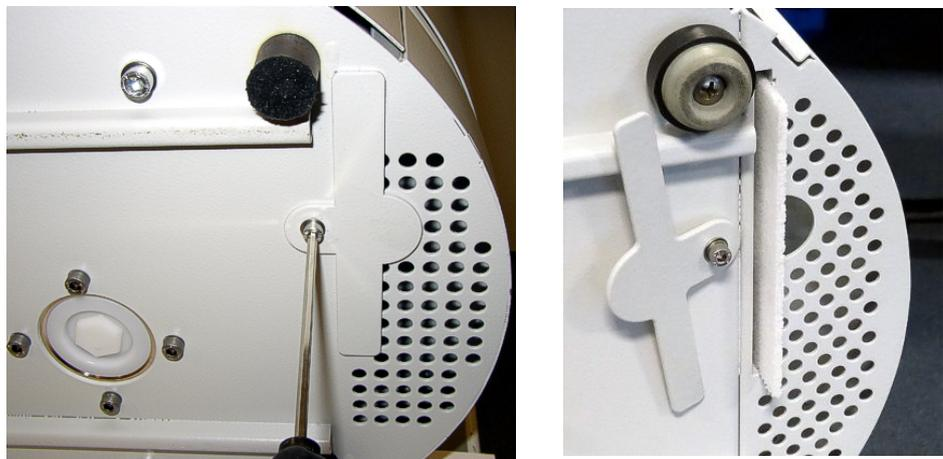
Fig. 46: Loosening the air filter cover
