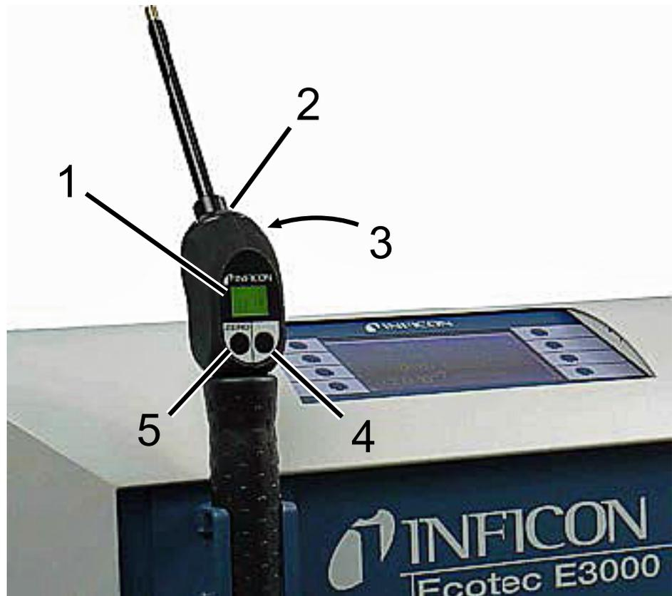
Fig. 4: Sniffer handle Display and functions
