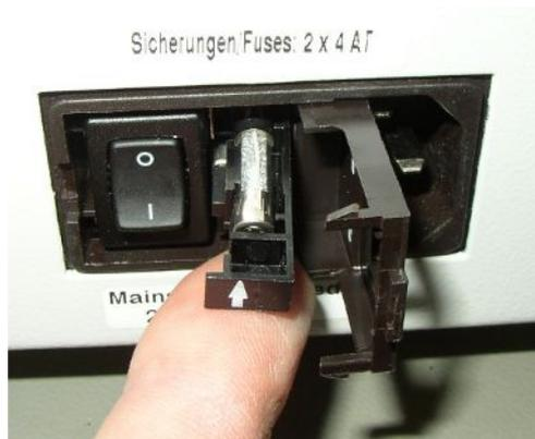
Fig. 51: Slot with fuse
