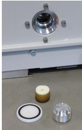
Fig. 48: Operating fluid reservoir open
