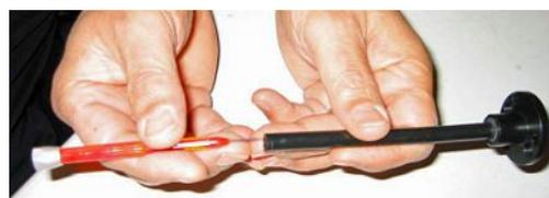
Fig. 7: Pushing out the capillary
