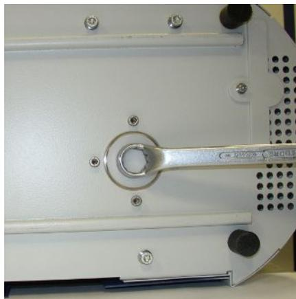
Fig. 47: Fastener of the operating fluid reservoir
