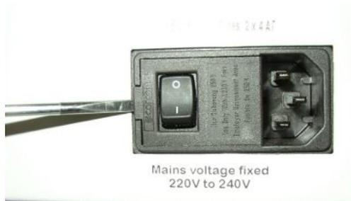
Fig. 50: Levering out cover to the right
