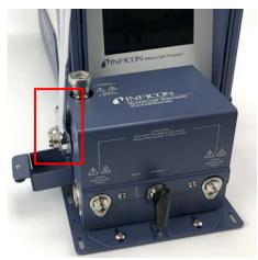
14 Cover the bonnet nut by reattaching the cover door using the thumb screw on the side of the device.
