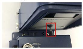
12 Loosely thread the front screws into the slide plate using a 3.0 mm hex driver.
