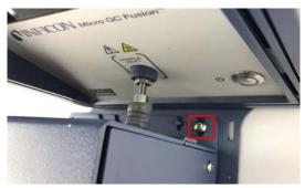
13 Tighten the transfer line nut to the front inlet of Micro GC Fusion one-quarter turn past finger-tight using a 5/16 in. wrench.
