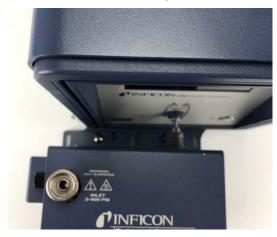
11 Gently push the device toward the instrument until the transfer line reaches the front inlet of Micro GC Fusion.
