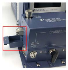
6 Using a 1 in. open-ended wrench, loosen the bonnet nut (PN 059-0809S) counter-clockwise.
