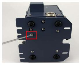
4 Attach the 1/16 in. sample transfer line with the rubber insulation sleeve onto the external sample conditioner using a 5/16 in. openended wrench.
