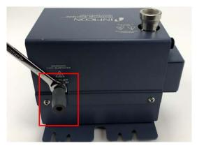
5 Slide the bottom mounting bracket underneath Micro GC Fusion and align the feet with the dedicated holes.
