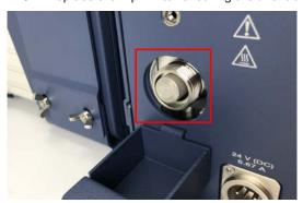
10 Re-install the bonnet nut and hand-tighten.
