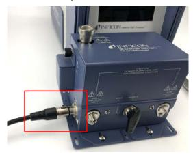
**20** Plug in the power cord to the power supply and connect to an AC power source.
