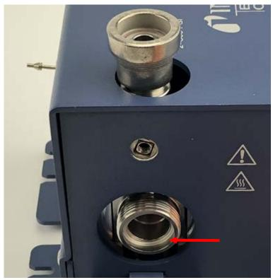
11 Replace the 7 µm filter ensuring the 7 is facing outward.
