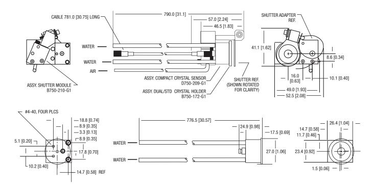
Feedthrough used for SL-A0E47, SL-A0E40, SL-B0E47, and SL-B0E40 sensor / feedthrough combinations (feedthrough PN 002-043) NOTE: Measurements in cm [in.]
