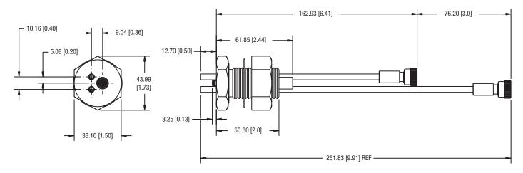
Feedthrough used for SL-A1E37, SL-B1E37, SL-A1E30 and SL-B1E30 sensor / feedthrough combinations (feedthrough PN 750-030-G1) NOTE: Measurements in cm [in.]
