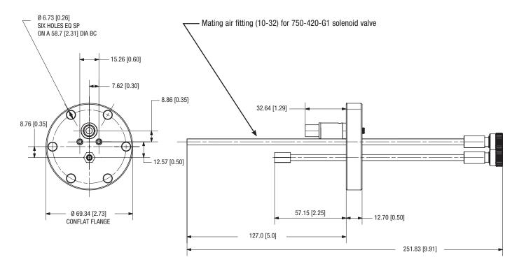
Feedthrough used for SL-A0E37, SL-B0E37, SL-A0E30 and SL-B0E30 sensor / feedthrough combinations (feedthrough PN 002-042) NOTE: Measurements in cm [in.]
