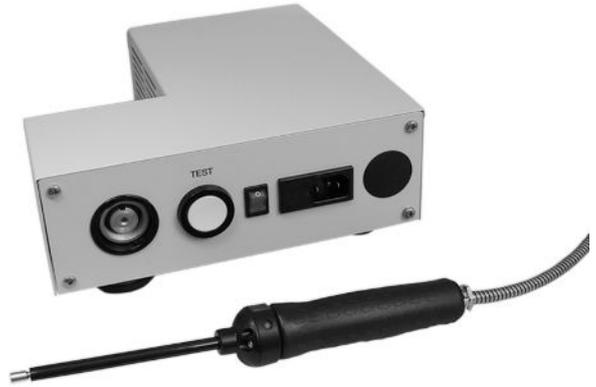
Helium sniffer QUICK-TEST QT100 with sniffer
