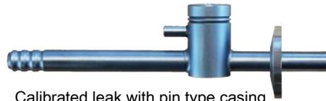
Calibrated leak with pin type casing
