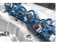
At the same time, the need for lower fuel consumption drives the use of high pressure fuel injection. Fuel leaks can negatively influence the fuel consumption and could cause a fire in the engine compartment. With increasing fuel injection pressures, larger leak rates will be generated by the same size leak.
