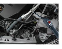
The Ecotec E3000 Multi-Gas Leak Detector is the only instrument available today that detects quantitatively refrigerant and fuel simultaneously—without false alarms from other materials (washer fluid, coolant, lock tight, etc). Ecotec E3000 can be set-up to detect up to four different gases at the same time, making it the
