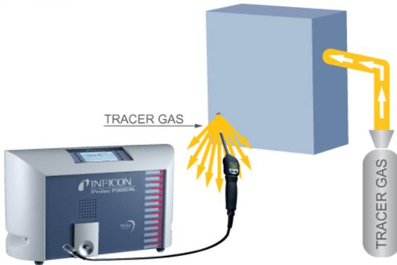
The fuel circuit of injection engines is tested via helium sniffing in production.
