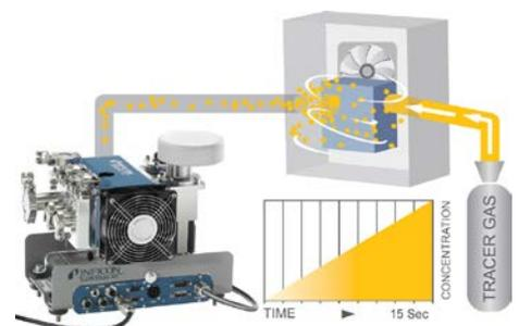
In accumulation testing, the motor housing is filled with helium, placed in an accumulation chamber and the rise in helium concentration in the chamber is detected by an [LDS3000 AQ leak detector](#).
