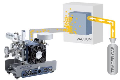
In vacuum chamber testing, the drive motor is filled with helium, placed in a vacuum chamber and any helium escaping from a leak is detected by the [LDS3000 leak detector](#).
