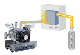
In vacuum chamber testing, the drive motor is filled with helium, placed in a vacuum chamber and any helium excaping from a leak is detected by the LDS3000 leak detector.
