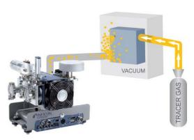
Battery cells prefilled with helium are typically tested via vacuum chamber leak detection. This process is very common for prismatic battery cells.
