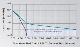
— conventional leak testers — UL5000 with HYDRO·S
