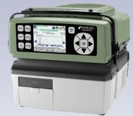
**Service Module:** allows for general maintenance and can be used as an alternate source of vacuum during stationary operation.
