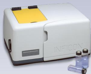
**HAPSITE HeadSpace Sampling System:** for highly accurate on-site analysis of VOCs in water, soil, and solids, with detection limits into PPT range.
