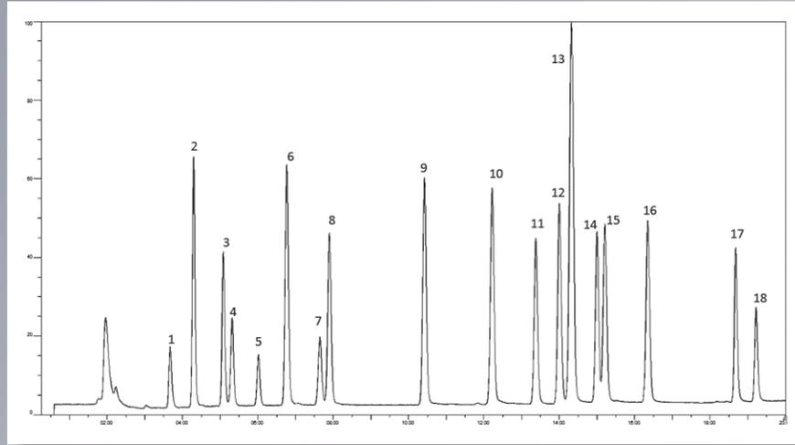
0.5 ppb nineteen commonly monitored VOCs in drinking water; temperature profile: 60.0°C (hold 1 min) to 90.0°C at 4.0°C/min, to 135.0°C at 6.0°C/min, to 200.0°C at 20°C/min (hold 45 sec)
