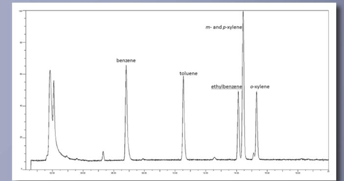
2 ppb BTEX; temperature profile: 60.0°C (hold 5 min) to 100.0°C at 25.0°C/min, to 120.0°C (hold 5 minutes) at 7.0°C/min
