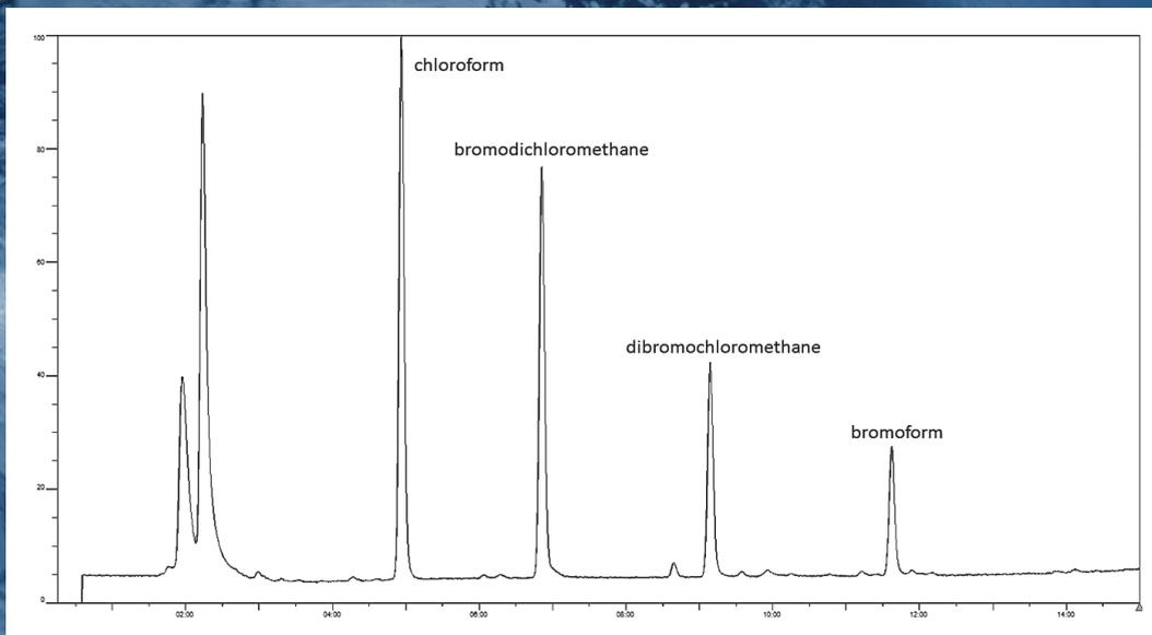
10 ppb disinfection byproducts-trihalomethanes (THMs); temperature profile: 55.0°C (hold 5 min) to 120.0°C at 6.0°C/min
