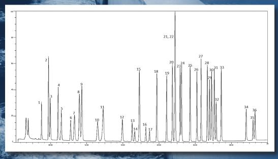
10 ppb thirty-six compounds from US EPA 624.1 Wastewater method; temperature profile: 50.0°C (hold 15 min) to 200.0°C (hold 2 min) at 6.0°C/min Column: DB-1, 30 m, 0.32 mm ID, 4.0 µm df
