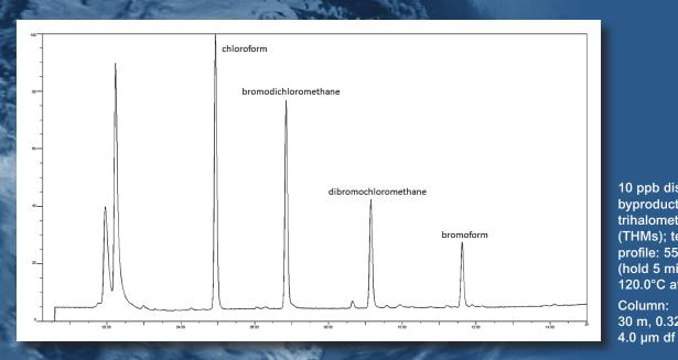
10 ppb disinfection byproducts-trihalomethanes (THMs); temperature profile: 55.0°C (hold 5 min) to 120.0°C at 6.0°C/min Column: DB-1, 30 m, 0.32 mm ID,
