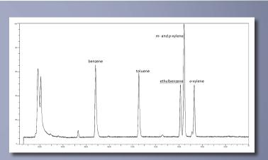
2 ppb BTEX; temperature profile: 60.0°C (hold 5 min) to 100.0°C at 25.0°C/min, to 120.0°C (hold 5 minutes) at 7.0°C/min
