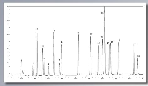
0.5 ppb nineteen commonly monitored VOCs in drinking water; temperature profile: 60.0°C (hold 1 min) to 90.0°C at 4.0°C/min, to 135.0°C at 6.0°C/min, to 200.0°C at 20°C/min (hold 45 sec)
