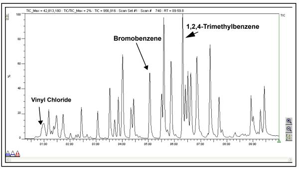
Figure 1: Example Chromatogram of the Analytes in the 524.2 Volatiles MegaMix with Gases
