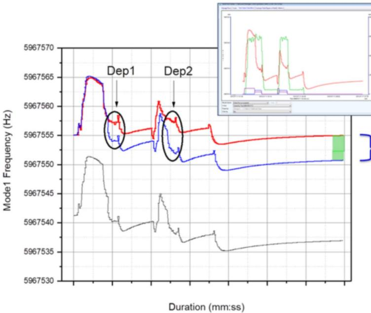
The difference between no Deposition (no net Frequency change in Hz from the start to finish of the wafer process) and normal Deposition (3-5Hz drop per wafer) is easily measured by the QCM with its resolution of 0.003 Hz
