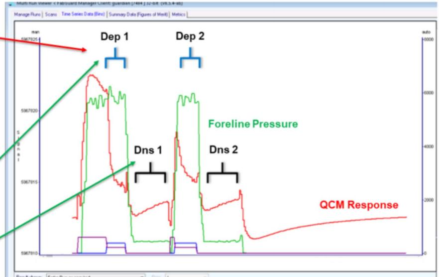
Dep = Deposition step where the TDMAT precursor flows and Deposits Titanium Nitride on the wafer Surface – Frequency Drop
