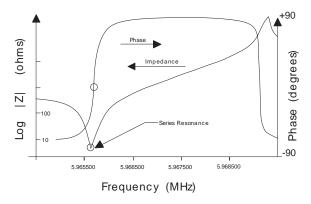
near the series resonance point, as shown in Figure 3. Oscillator circuits are normally designed so that the crystal is required to produce a phase shift of zero degrees, forcing the circuit to operate at the crystal's series resonance frequency.
