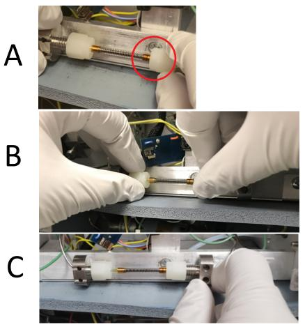
**9** While holding the right concentrator elbow in place with your fingers, insert and tighten the bottom screw until finger tight. Continue to stabilize the right concentrator elbow in place with a 3/8" wrench, insert the top screw and evenly tighten the screws until snug. Do not overtighten. Overtightening will cause the elbow to turn. See Figure 11.
