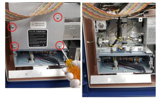
Figure 4 Remove four screws and upper oven cover
