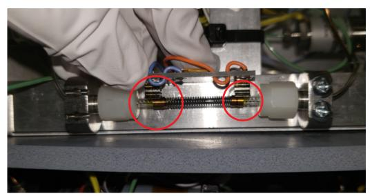
**12** Press the concentrator board gently but firmly onto the concentrator. See Figure 14.
