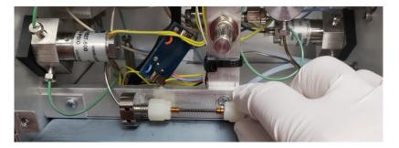
**6** Using a 3/8" wrench, stabilize the concentrator elbow on the right side. Using a screwdriver, unscrew and remove the two screws that hold the elbow in place. Retain the screws for use when reinstalling. See Figure 7.
