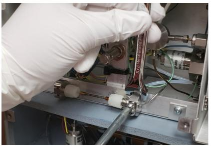
**7** Gently remove the concentrator from the concentrator elbows. See Figure 8. *Figure 8 Remove from the concentrator elbows*
