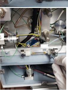
**11** Line up the clips from the concentrator board with the metal contacts on the concentrator. See Figure 13.
