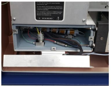
**3** Unscrew and remove the four screws that hold the upper oven cover in place. Retain the screws for reuse. Remove the upper oven cover. See Figure 4.
