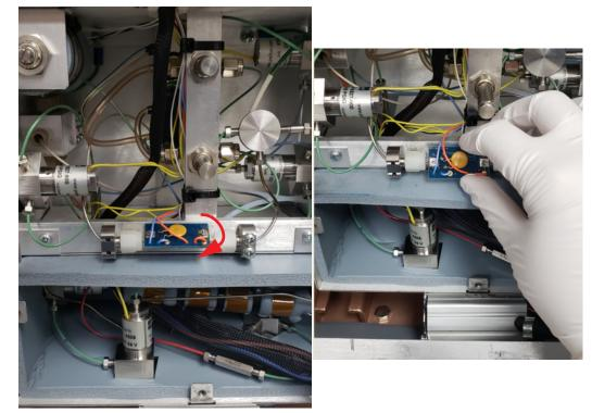
**5** Using a 7/16" wrench, loosen the nuts on each side of the concentrator by 1/4 of a turn. Loosen the nut on the right side upwards and the nut on the left side downwards. Using fingers, fully loosen both ends of the concentrator. See Figure 6.
