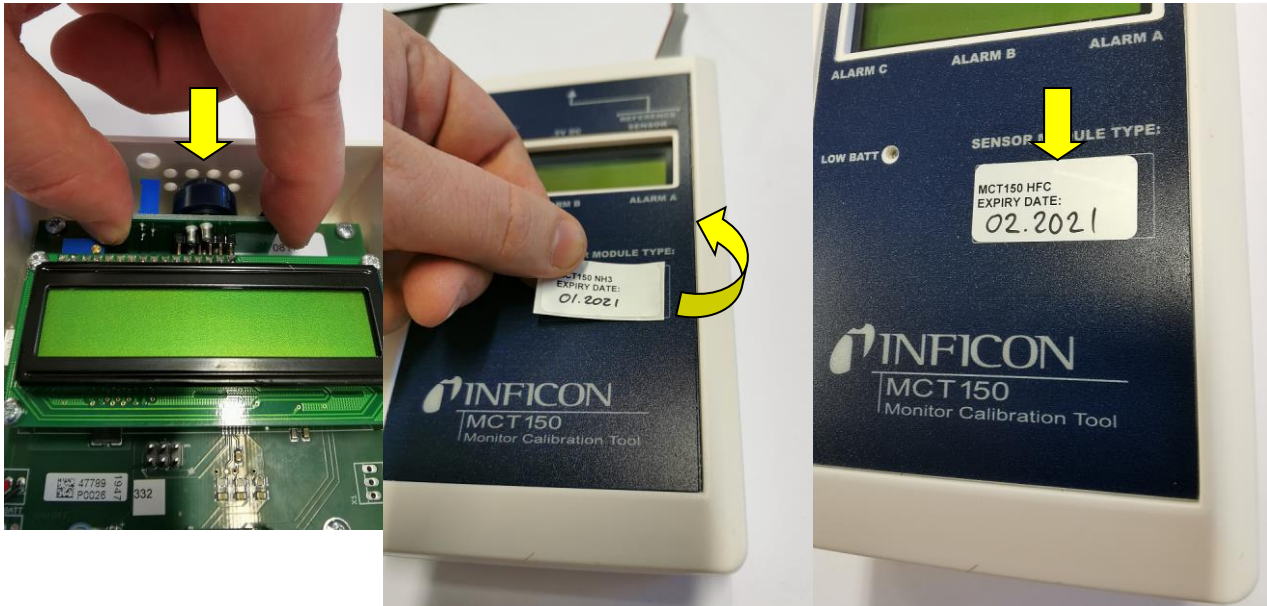
4. Mount the sensor module in the plug-in socket
